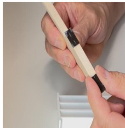
5. Position the mounting tool flush with the rear edge of the black keyboard key (1). Insert the RR Janko® key from above (2), making sure it does not stick to the sides of the mounting tool and align with the rear edge of the mounting tool (3). Now guide it straight down in parallel and press firmly (4) to ensure full adhesive strength.
